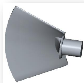
Pale de turbine impression 3D/PETG
